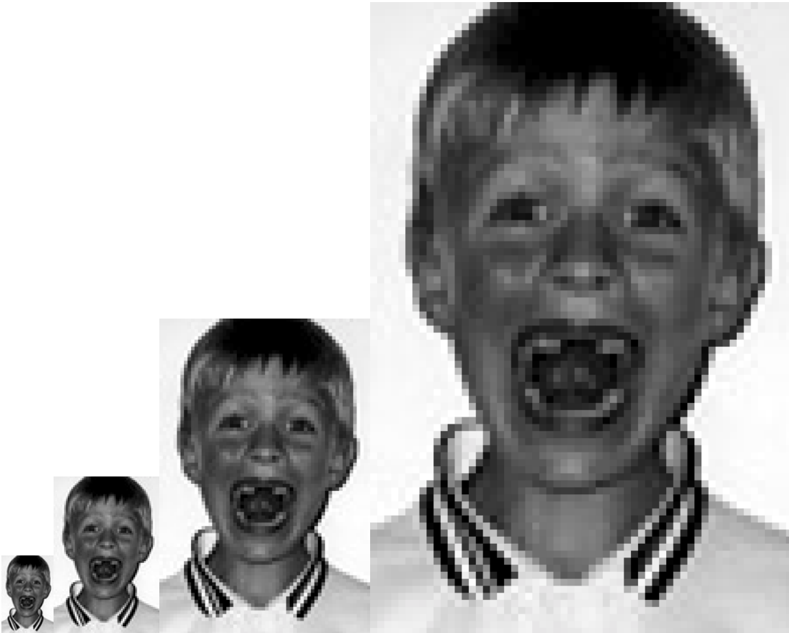
Figure 21 – The image on the left is a 150-dpi, 8-bit grayscale scan. The spatial resolution is appropriate for its size. The next image was created by enlarging the first. Its resolution is now 75 dpi. The third image is enlarged even further and is now 37.5 dpi. The last image is 18.75 dpi.
