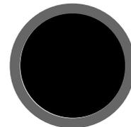
*Figure 1 - The mark made by a single laser spot. The gray area around the laser spot signifies the variation in size that may occur due to changes in exposure or processing conditions. (Note: Individual laser spots may not be perfectly round as shown here.)*
