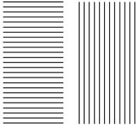
Figure 2 - Extremely narrow horizontal and vertical lines are used as a test target for automatic calibration.
