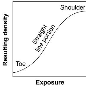
Figure 2 - Generic characteristic curve showing toe, straight line portion, and shoulder.
