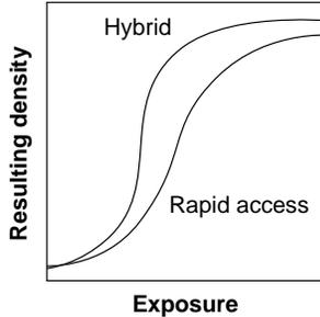
Figure 3 - Generic rapid access film versus a generic hybrid film.
