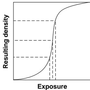
Figure 6 - Slight changes in exposure on a very high contrast film may cause large changes in dmax.
