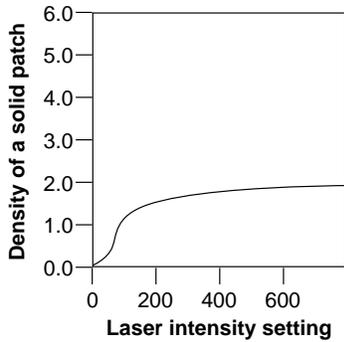
Figure 5 - Characteristic curve of a rapid access paper as output on a Linotronic 330. Note the low dmax.
