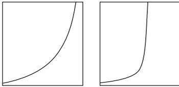
Figure 7 - A broad curving toe (left) indicates a film with less edge sharpness than one with a rapidly curving toe (right).
