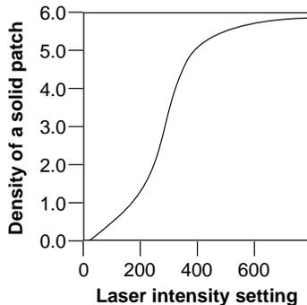
Figure 4 - Example of a characteristic curve of a rapid access film as output on a Linotronic 330.
