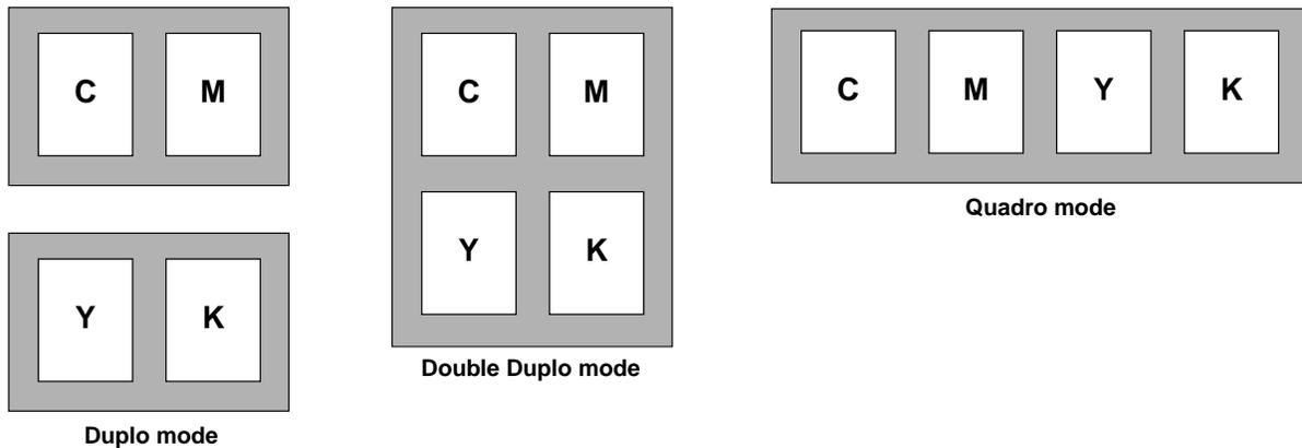
Figure 3 - Duplo mode, Double Duplo mode, and Quadro mode are all ways of maximizing film use with Automatic Page Positioning with Linotype-Hell Production Tools..
