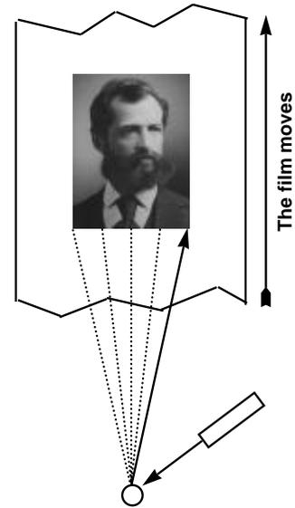
Figure 1 - With a capstan device, the optical system remains stationary, and passes a laser beam across a moving piece of film.
