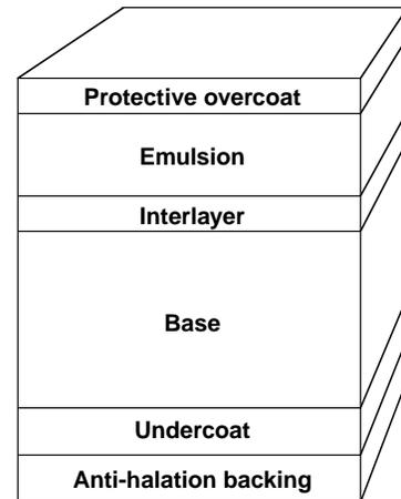
Figure 1 - Cross section of a typical graphic arts film.
