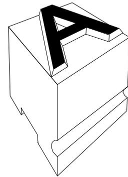
Figure 1 - A single cast letter from a hot metal font.
