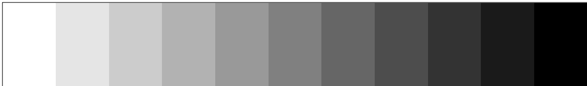
Figure 1 - Dot percent scale from 0% to 100% in 10% steps at a coarse screen ruling.
