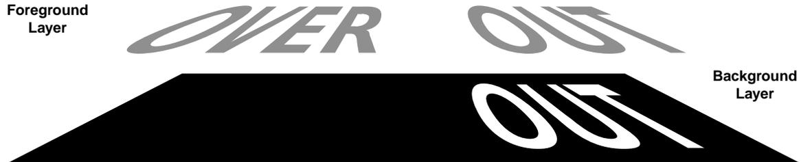
Figure 3 - An overprint (left) and a knockout (right) shown as two layers.
