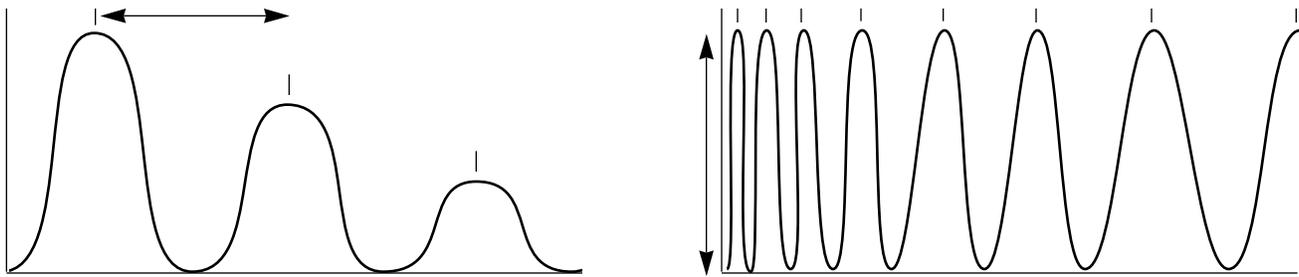
Figure 3 – An amplitude modulated wave form (left), and a frequency modulated wave form (right). The amplitude modulated wave varies in height. With the frequency modulated wave the height (i.e., the amplitude) is constant but the frequency varies.
