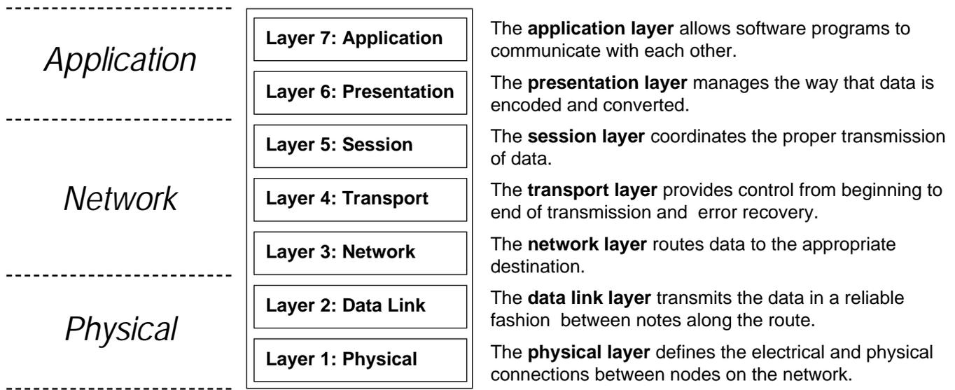
Figure 3 – The different layers of the OSI standard define how communication is maintained between network users.
