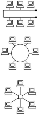
Figure 2 – Network topologies: bus (top), ring (center) and star (bottom).
