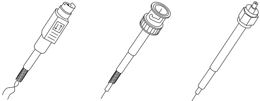
Figure 1 – Three examples of the most common guided media: LocalTalk shielded twisted pair with a DIN 3 connector (left), Thinnet coaxial with a BNC connector (center) and fiber optic cable with a Type 906 connector (right).
